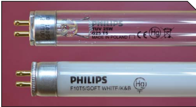
FIGURE 4. UV-C lamp (top) and fluorescent lamp (bottom) of the same form factor, which could be made on same lamp machine. The UV-C lamp has a fused quartz envelope that is clear in order to let UV-C light through unfiltered. The fluorescent lamp glass envelope is lined internally with phosphor, which glows when charged. (Image courtesy of UV Resources.)
